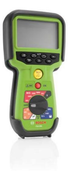
The FSA 050 is an important and simple diagnostic module for testing vehicles with electric and hybrid drive. With the ability to work wirelessly it's capable of performing multimeter functions such as voltage, resistance, capacitance, insulation and continuity tests, with measurements on the high voltage side up to 600 V (CAT IV1) as well as testing insulation resistance up to 200 GOhm at test voltages of 50 to 1,000 V.
