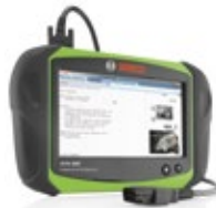
KTS 350 Compact all-round solution for comprehensive vehicle diagnostics
